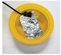
**4** — Unfold the wire screen to a 90° angle, leaving the foil barrier strip in place on the screen. Insert the screen into the bowl of the yellow base with foil side pointing up. Place the creen so that it will be about parallel with and clear of the bulb/socket
