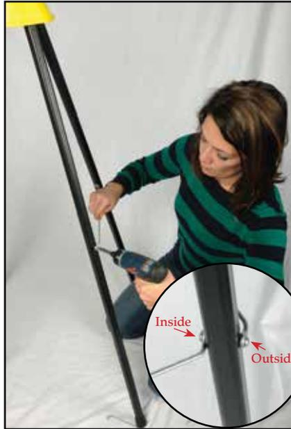
3. Screw metal brackets into legs. Two brackets will fit on the outside of legs and two will fit on the inside of legs. **Note: Make sure to position holes as indicated in photo above.**
